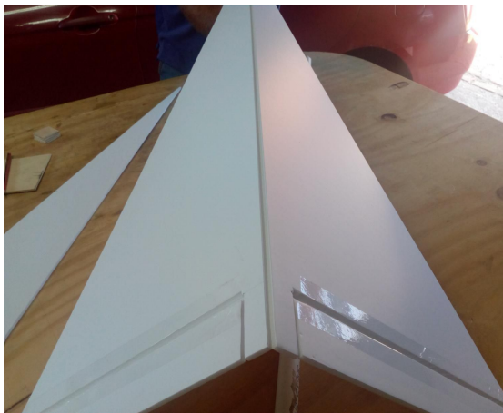
8 Above: With wing bottom up, cut along the centre line but not right through.
